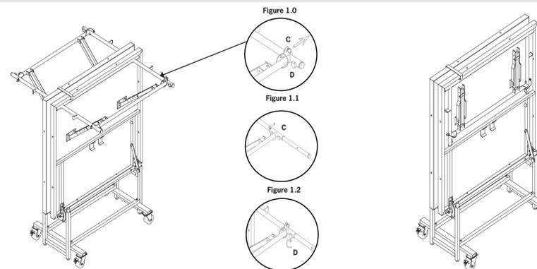
7. Fold down legs on both sides of the stage. Your stage is now ready for storage. You can roll the stage to your desired storage location. Once it is at your desired location engage the breaks on the casters with your foot, so the stage stays stationary
