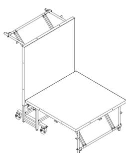
3. Loosen knob I and reposition safety bar F by moving it downward and connecting it to knob G. Tighten knob G (see Figure 1.0 to 1.2)
