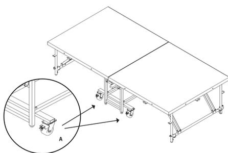
1. Engage breaks on both casters by pressing brake lever A down with your foot, so that the stage cannot move
