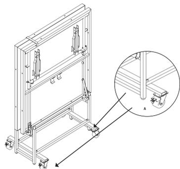
1. Roll the stage to the location you would like to set it up. Engage breaks on both casters by pressing brake lever A down with your foot, so that the stage cannot move
