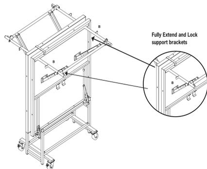
2. Unfold legs on both stage half platforms. Make sure the leg's support brackets are fully extended and locked
