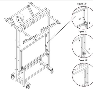
4. Remove safety bracket E from the top of the stage
